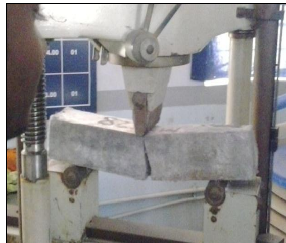
Fig. 3: Flexure Strength of Concrete.
